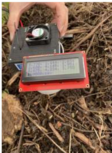
Figure 2. Electronic nose in compost.
